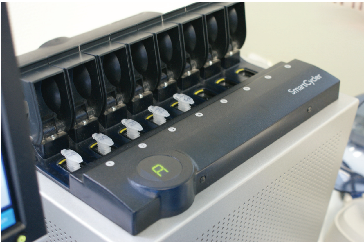
Figure 1. Smart Cyciler equipment, where DNA amplification is performed and the results are analyzed
